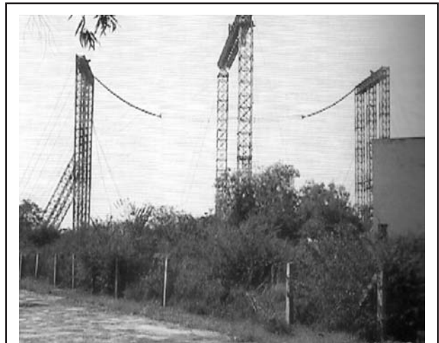
Fig.9: A view of mock up test facility showing two and the divider dead end and central portal tower
